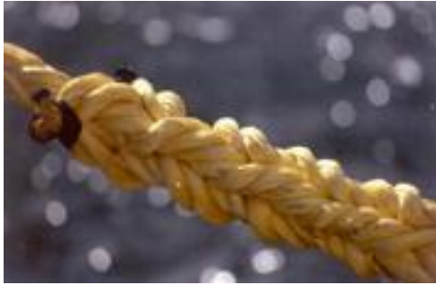
Rope in good condition
