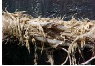
Rope in bad condition
