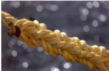
Rope in good condition
