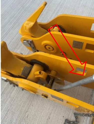
Fig 4 Release Position push back
