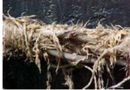
Rope in bad condition
